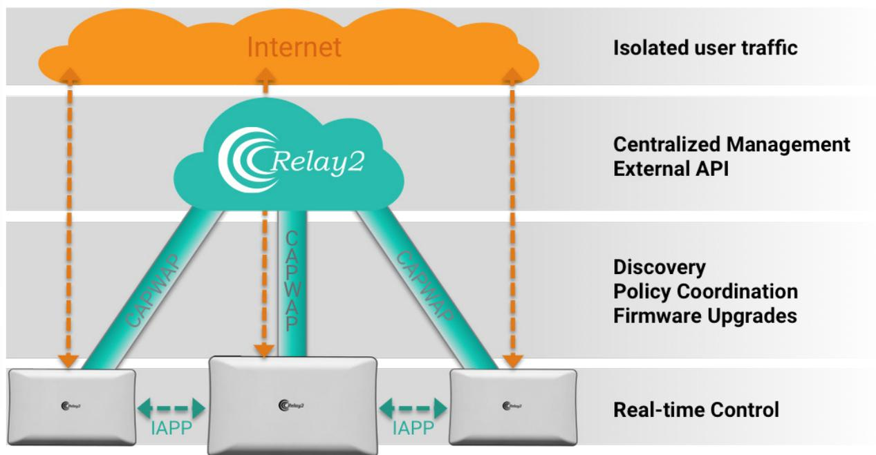
Figure 2: Relay2 Cloud Wireless Networking Architecture
