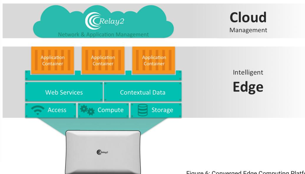
Figure 6: Converged Edge Computing Platform
